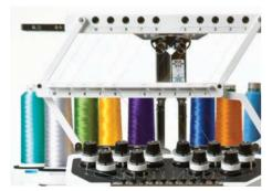
Flexible threading system Easy threading prevents thread tangles and knots and provides stable thread tension.
