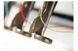
Automatic needle threading Simply press the automatic needle threading button and the upper thread will pass through the needle. It couldn't be simpler.
